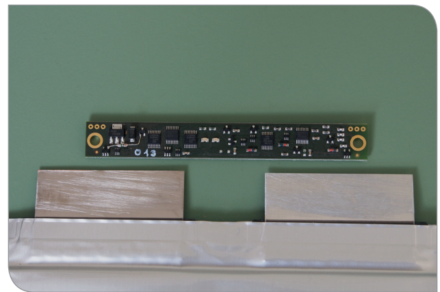
Prototype of a board for battery monitoring on cell-level
